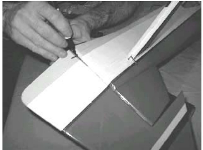
Insert pins on the centerline of each hinge to prevent them from sliding too far in. Install the hinges, rudder and tiller arm.
