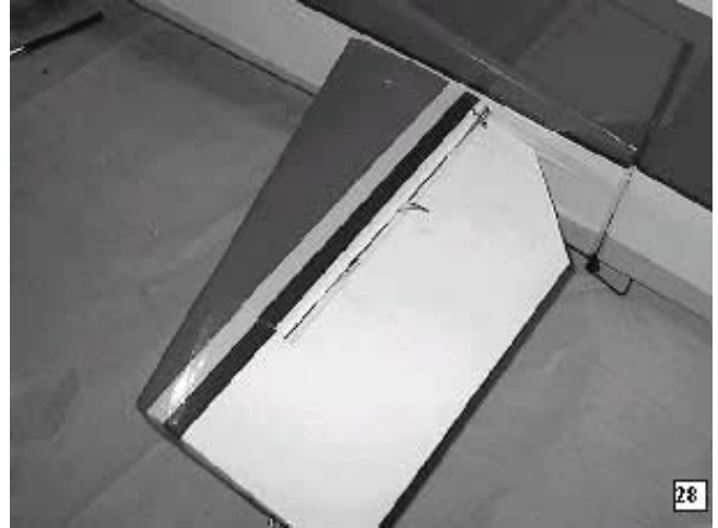
Use a toothpick to coat the inside of the hole with epoxy.
