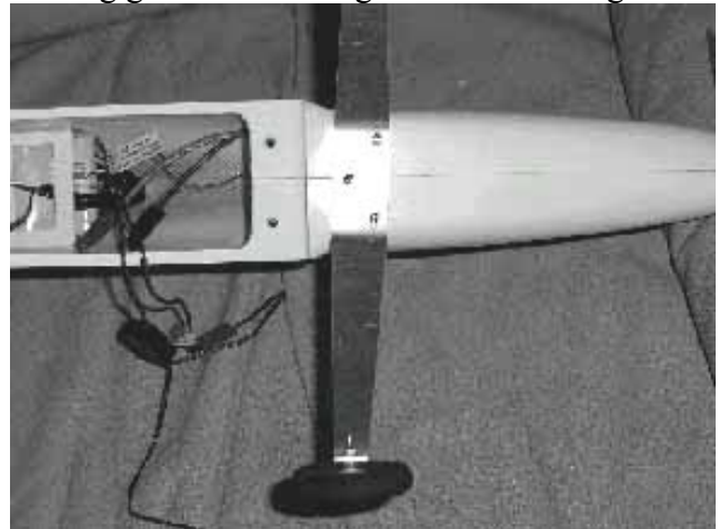
It is now time to set all the control throws. The elevator should have 3/16-inch travel up and down. The rudder should have 3/4-inch right and left. Ailerons should have 3/16-inch up and down. WARNING! Too much travel will cause uncontrollable snap rolls.
